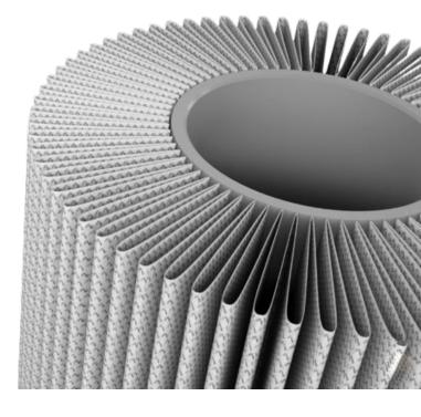
PP95BL cartridges consist of: 3-layer polypropylene filtering septum supported by an external PP drainage net and an internal PP drainage net (5 Layers filtering system); internal support and moulded rigid polypropylene terminals. The external drainage net of the 5 Layers filter system prevents the crease from closing due to the increase in pressure due to the dirty filter material, always ensuring the constant outflow of filtered water towards the internal support of the cartridge.
