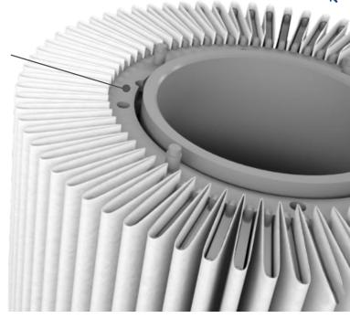
The FilterBig TPL95BHF cartridges consist of: moulded rigid internal support, moulded rigid polypropylene terminals and TekBlue pleated polyester mesh filtering panel coupled to a PP drainage net. The two nets are always kept perfectly open and in place by a special rigid polypropylene structure: the system filstar@inside
