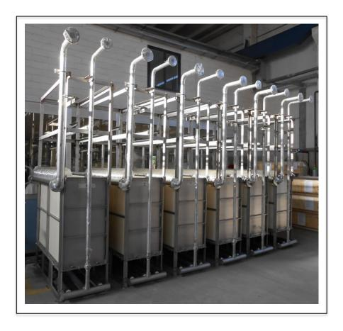
**PRODUCT TMR090-100S** N. MODULES 6 (Total 54 m<sup>2</sup>/h) 12 m<sup>3</sup>/h FLOW RATE WASTE WATER **CIVIL** WATER USE **SEWAGE DISCHARGE** OEM **Confidential (Italy) END USER Confidential (Australia)** SECTOR **MUNICIPAL**
