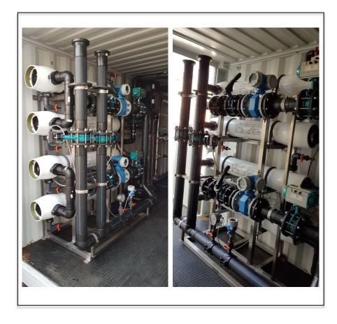
**PRODUCT FILTERBLUE-BL-03 FLOW RATE**  $144 \text{ m}^3/\text{h} (4 \times 36 \text{ m}^3/\text{h})$ WATER **SEA APPLICATION RO PRETREATMENT** WATER USE **INDUSTRIAL** OEM **Confidential (Italy) END USER Confidential (Italy) SECTOR REFINERY**
