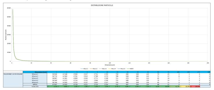
From this result it would seem that there are many small and less and less particles with larger diameters, with a curve similar to a hyperbola.
