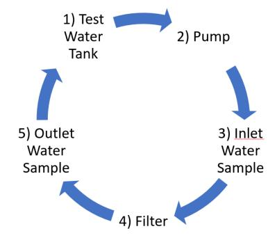
The water inside the tank is mixed with powders with a specific particle size. The water will then be pressurized by the pump through the filter, returning inside the tank.
