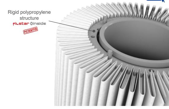
The FilterBlueMaxi TPL95BL cartridges consist of: moulded rigid internal support, moulded rigid polypropylene terminals and TekBlue pleated polyester mesh filtering panel coupled to a PP drainage net. The two nets are always kept perfectly open and in place by a special rigid polypropylene structure: the system firstar@inside
