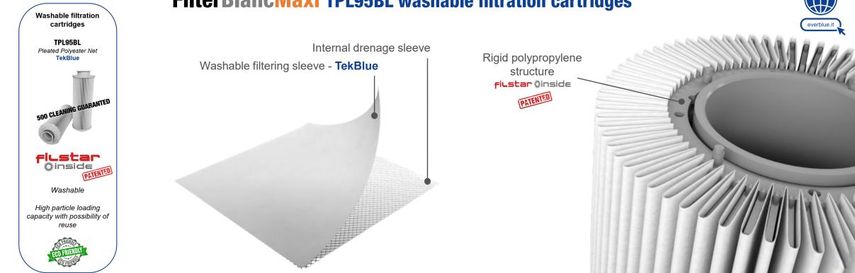
The FilterBlancMaxi TPL95BL cartridges consist of: moulded rigid internal support, moulded rigid polypropylene terminals and TekBlue pleated polyester mesh filtering panel coupled to a PP drainage net. The two nets are always kept perfectly open and in place by a special rigid polypropylene structure: the system **filstar** (inside
